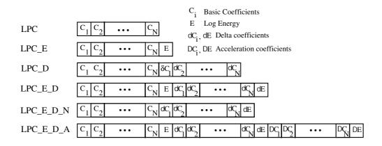
Fig. 5.5 Parameter Vector Layout in HTK Format Files
