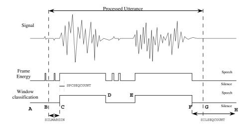
Fig. 5.6 Endpointer Parameters
