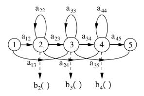
Fig. 7.1 Simple Left-Right HMM
