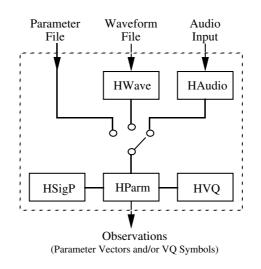
Fig. 5.1 Speech Input Subsystem
