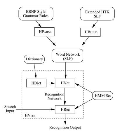
Fig. 12.1 Overview of the Recognition Process
