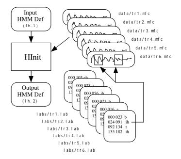
Fig. 8.4 File Processing in HInit
