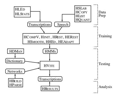
Fig. 2.2 HTK Processing Stages
