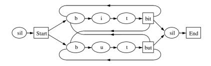
Fig. 12.8 Monophone Expansion of Bit-But Network
