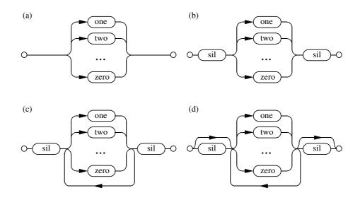
Fig. 12.4 Example Digit Recognition Networks
