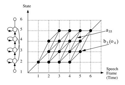
Fig. 1.6 The Viterbi Algorithm for Isolated Word Recognition
