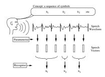
Fig. 1.1 Message Encoding/Decoding
