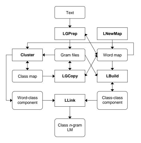
Fig. 14.2 The main stages in building a class-based language model
