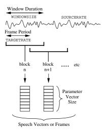
Fig. 5.2 Speech Encoding Process
