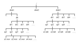
Fig. 6.2 Database Hierarchy: Data [Left]; Labels [Right].
