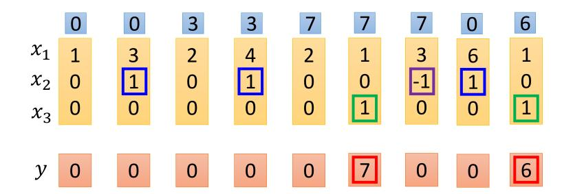
When  $x_2 = 1$ , add the numbers of  $x_1$  into the memory When  $x_2 = -1$ , reset the memory
